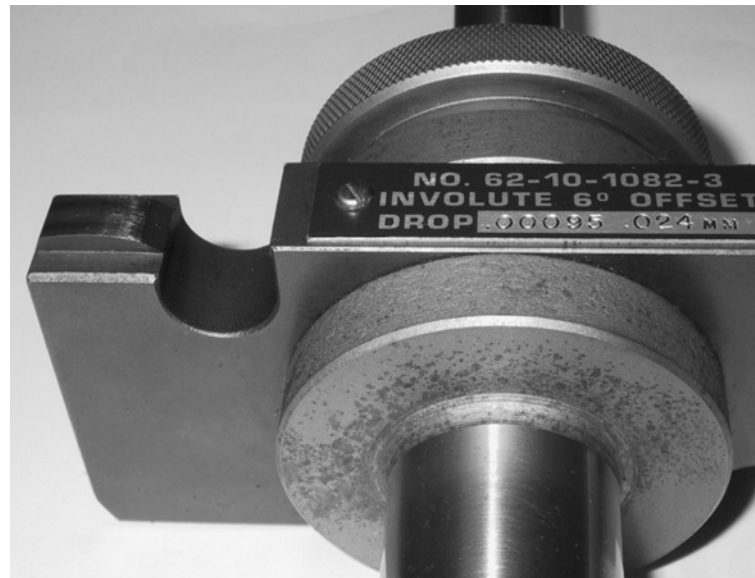
Figure 3 — 115 mm base circle diameter involute artifact
