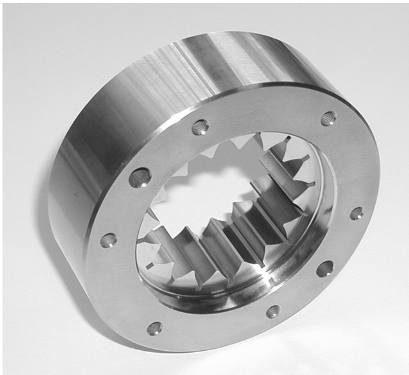
Figure 7 — Internal gear artifact
