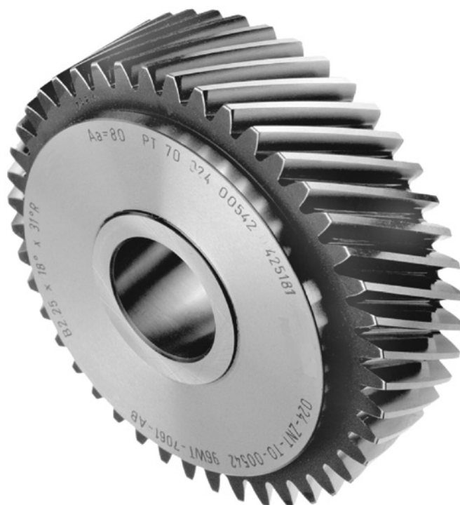
Figure 6 — Master gear artifact
