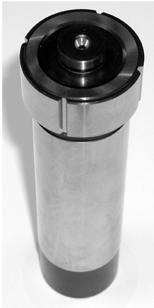
Figure 8 — Tooth thickness artifact
